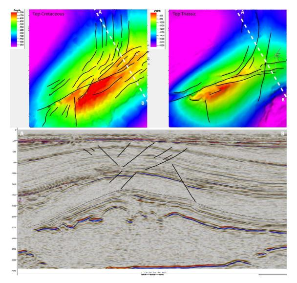
*Top left figure*: Top Cretaceous depth map with faults indicated by black lines. *Top right figure*: Top Triassic depth map and faults. The tiny grey lines in the middle right section of the figure indicate the trajectories of the VE-wells and TR-wells into the Zechstein salt formation below the Triassic formation.
